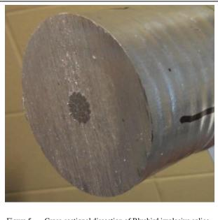
Figure 5. Cross-sectional dissection of Bluebird implosive splice.
