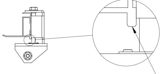
Shown here is an example of a groove that will prevent the WEEB teeth from properly penetrating the module frame. This type of frame is not compatible with the WEEB.
