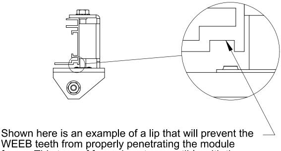
WEEB teeth from properly penetrating the module frame. This type of frame is not compatible with the WEEB.
