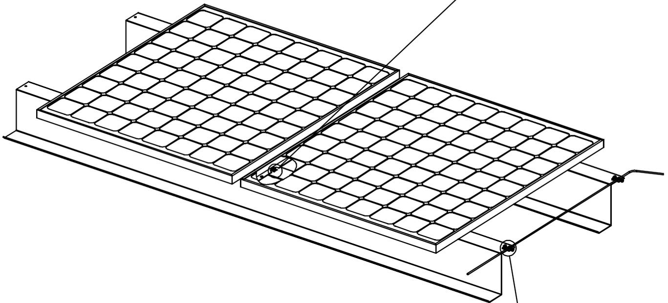
Drill bolt clearance hole  $\text{Ø}17/64\text{in}$  [7mm] on center of rail. Assemble WEEB-LUG-6.7 assembly and torque fasteners to 10ft-lb / 13.5N-m using Penetrox-A on threads.
