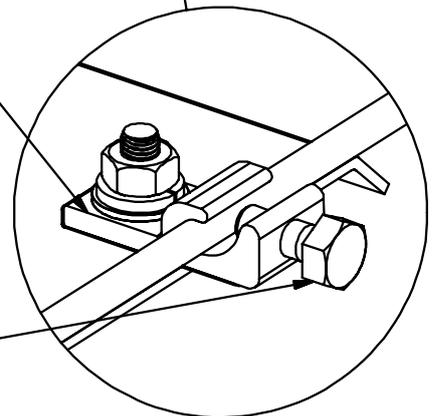
Lay in equipment ground conductor and torque bolt to 7ft-lb / 10N-m
