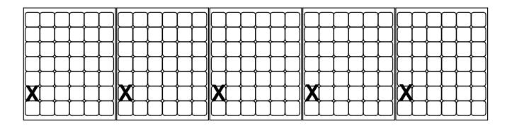
One WEEB-DSK14 or WEEB-UIR is to be installed on each module
