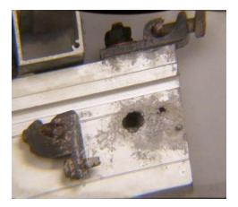
Nearly all grounding devices used to establish a ground bond to aluminum module frames incorporate a stainless steel to aluminum connection. Proper installation of these devices makes a huge difference in their long-term performance. Selecting the right device for use in a corrosive environment can make a large impact on the longevity of the system.
