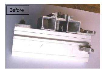
Corrosive atmosphere tests are an absolutely crucial part of evaluating grounding and bonding devices. The ASTM B117-09 salt fog test is a good starting point for corrosion testing of grounding and bonding connections. To truly test the corrosion resistance of the WEEBs, a more rigorous test was performed as part of their development. This test subjected a WEEB, a WEEB Lug, and a traditional lay-in lug (installed
