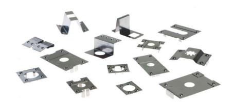
self-retain to form a connection that is highly resistant to oxidation and galvanic corrosion. The action of the WEEB teeth embedding and deforming to create such a connection necessitates that the WEEBs be a one-time use part. The same degree of protection cannot be reached by a device that is allowed to be used multiple times.
