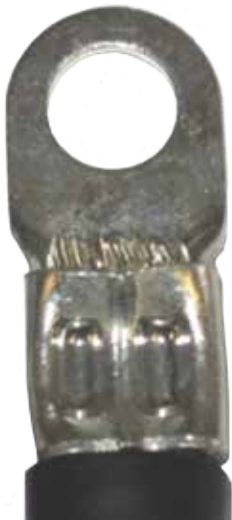
Close up of "M" Profile Crimp
