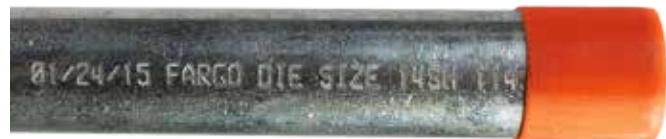
Above: close up of marking on Fargo splice requiring 14SH die index.
