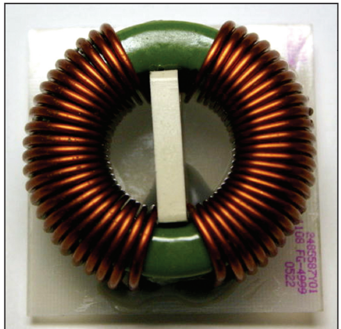
Fig. 7. The new wire-forming technology allows a common-mode inductor to be wound easily on a single toroid with gaps.
