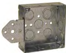
"B" Bracket Face mounts on front edge of wood stud. Use when space between studs is limited.
