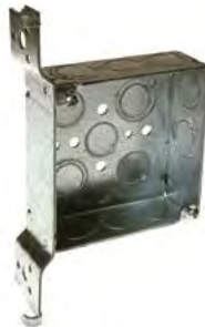
BOX-LOC® "MS" Bracket Positions box on either side of stud. BOX-LOC® (MS) Bracket Box is a snap to install. Place the bracket on the open side of the stud first. Slots in the bracket engage the lip of the stud and actually crimp it as you press the bracket on the stud. Barbed hooks dig into the flat side of the stud, quickly locking it into place.
