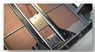
Cover is then rotated 90 degrees and the test is repeated (side impact)
