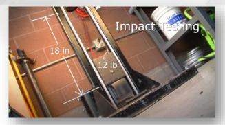
Cover/Hinge must pass a 12 LB weight dropped at a height of 18 IN
