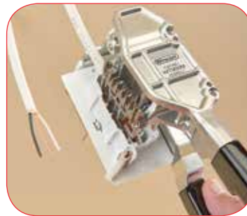
3 Squeeze handles together to terminate cable.
