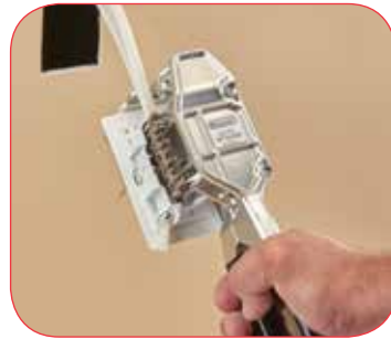
5 Squeeze handles to terminate second cable.
