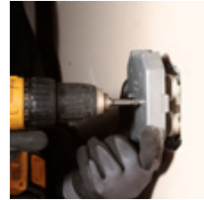
4. Remove cover by removing the mounting screws.
