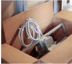
1. A protection plate can be added to prefabricated assemblies to protect wiring and devices during shipping and handling.
