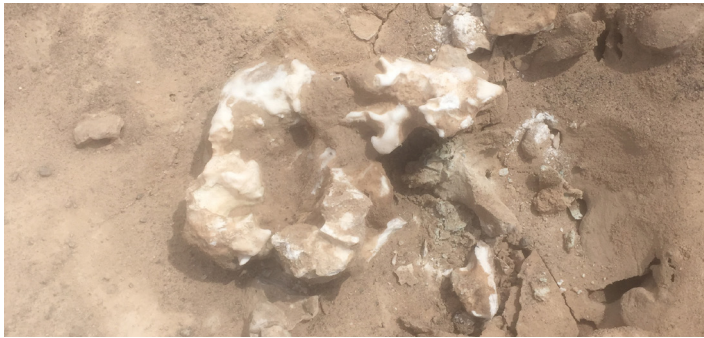
The Caliche can best be described as salt-cemented sand. It is very dense and hard.
