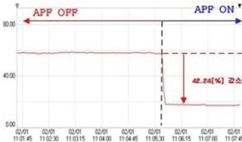
Figure 8: THDi at panel 2AHF-2A reduced from 59.60% to 17.36%
