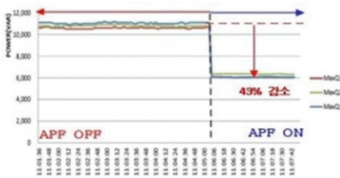
Figure 12: Reactive power at panel 2AHF-2A reduced 43% from 10.8 kvar to 6.1 kvar
