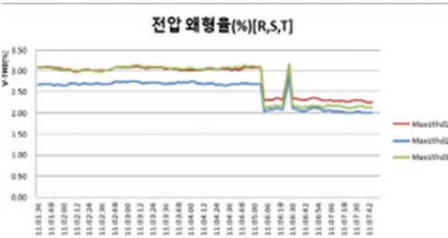
Figure 9: THDv at panel 2AHF-2A reduced by 16%
