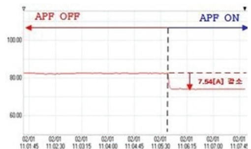
Figure 10: Load current at panel 2AHF-2A reduced from 83.12 A to 74.58 A
