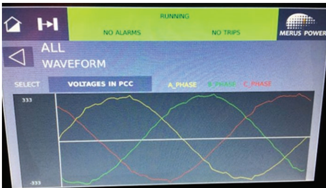
Figure 7: HMI showing voltages at 2AHF-2A panel
