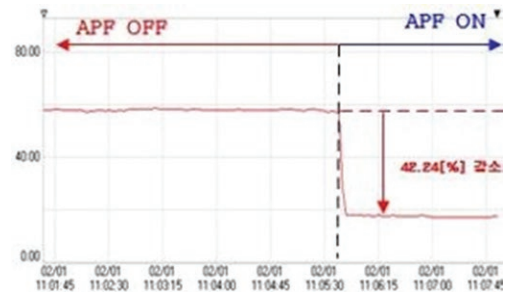
Figure 8: THDi at panel 2AHF-2A reduced from 59.60% to 17.36%
