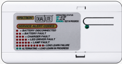
External PUSH TO TEST switch, AC ON indicator and Spectron® Self-Test/Self-Diagnostics are standard
