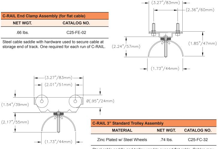
Steel cable saddle and trolley used to support flat cable. Cables may be stacked in saddle.
