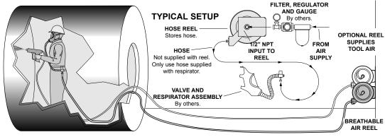
FIGURE CLEAN AIR REELS include stainless steel air path. Also includes ball stop and ratchet lock. Finish is OSHA safety blue baked-on polyester. 3/4"-16 UNF fitting to fit MSA #455022 hose or equivalent. Does not include hose.
