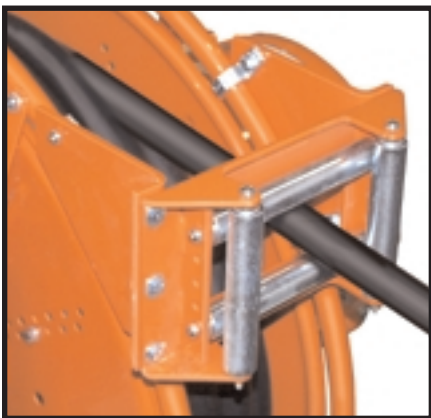
Cable guide with nylon or steel rollers (optional) clamps to hoop guides and may be adjusted throughout entire circumference of hoop.
