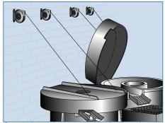
Sound dampening covers on vibrating cleaners make sound level in a metal finishing plant more acceptable. Two RETRIEVERS lift part of each cover's weight and make opening easier and safer.
