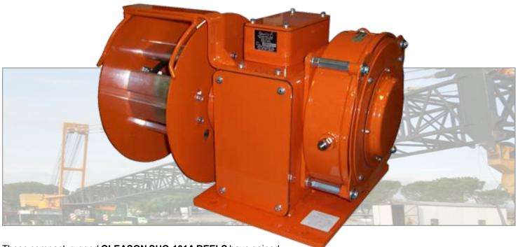
These compact, rugged **GLEASON SHO-101A REELS** have gained much favor with the scrap handling industry and manufacturers of magnet handling cranes. Designed to fit within the crane boom, it is the answer to magnet cable handling problems. Constructed entirely of steel with a powerful long-life main spring. Precision ball bearings are used throughout. Heavy cross section slip rings and coppergraphite brushes ensure electrical contact. Collector assembly rating - 2 pole, 75 amp, 600 volts.
