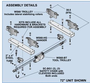
Heavy Duty Rolling Rail mounts in two parallel rails, which must be supported every 6' (1.8m) to maintain rated capacity. Recommended distance between support rails is length of tool rail less 12" (305mm). **MAXIMUM RATED CAPACITY OF ROLLING RAIL** includes tool, balancer, and attachments.
