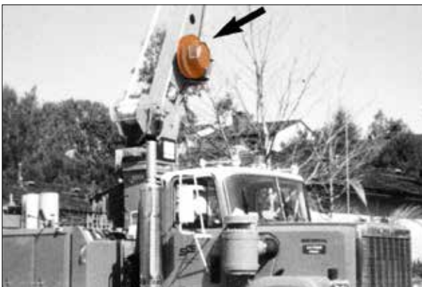
GLEASON K-REEL installed on a hoist.
