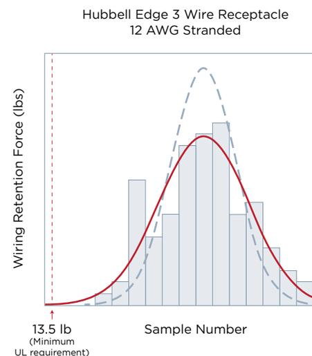
When compared to the minimum requirement for wire retention, Twist-Lock Edge screwless termination offers superior strength.
