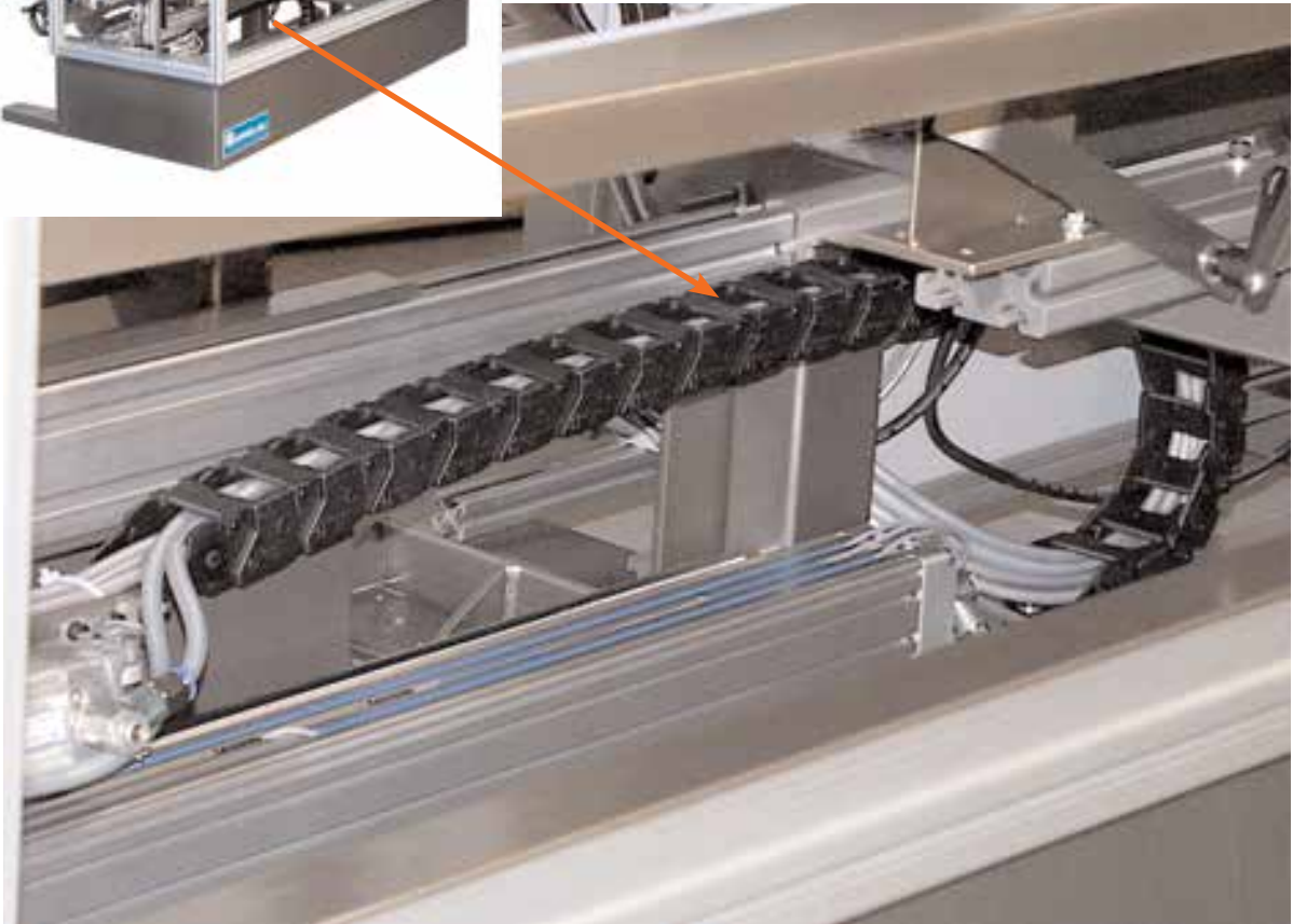
Type GRP PowerTrak protects power cable and allows unhindered movement on case erecting machine.
