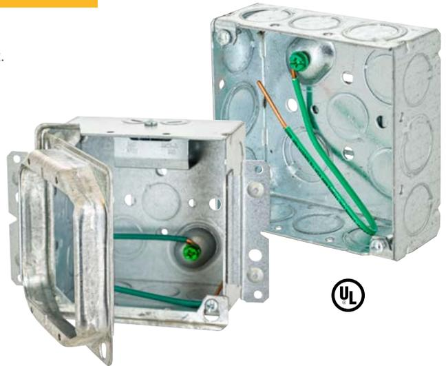
**Boxes -** 4" Square, 2-1/8" deep. **Construction -** Welded steel with raised grounds. **Capacity -** 30.3 in.<sup>3</sup>
