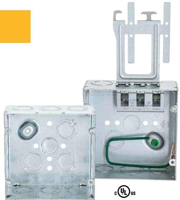
**Boxes** - 4-11/16" Square, 2-1/8" deep. **Construction** - Welded steel with raised grounds. **Capacity** - 42 in.<sup>3</sup>
