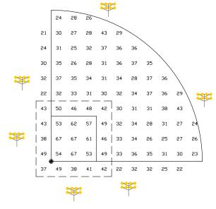
Fixture: 740W Turf Fixture Count: 44 Average Light Level: 50fc (infield) 30fc (outfield) Total Wattage: 32,560 W
