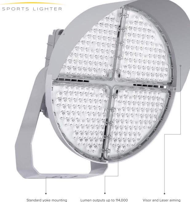
Standard yoke mounting with single 3/4" bolt. Yoke also includes vertical aiming indicators, adjustable in 5 degree increments. Fixture is 3G vibration rated. Lumen outputs up to 114,000 lumens and 153 LPW give superior performance to legacy products and provide additional energy savings.
