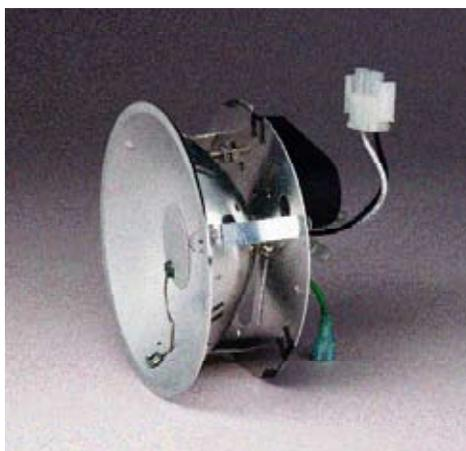
A polished anodized reflector for the bi-pin lamps have an adjustable socket to change the light distribution. A glare shield is standard.
