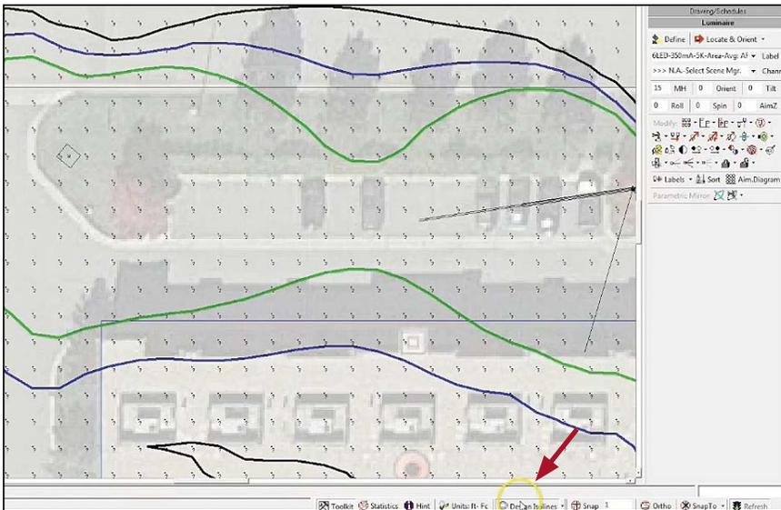
(63) But they can be turned on simply by clicking the Design Isolines button at the bottom right hand side of the screen.
