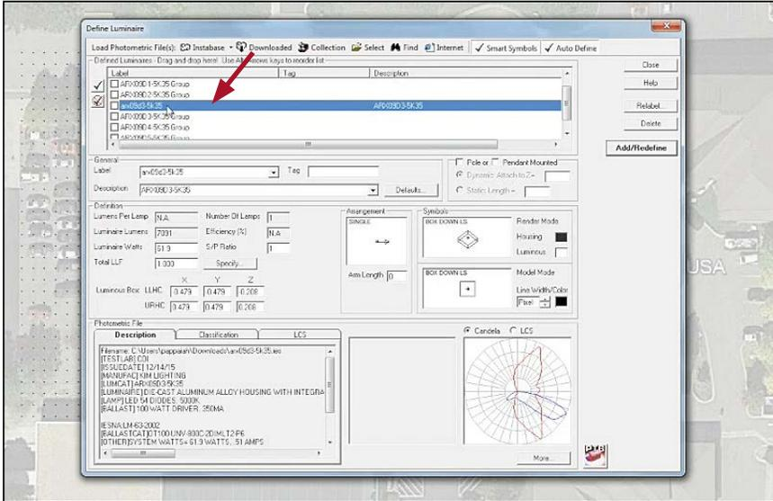
(24) Also notice the composite IES file that we imported from the website and it's corresponding group file. As you can see when clicking on them, you can tell the difference between the two because the "Group" file has an orient and tilt associated with it and the composite file does not. Also, the group files have the word "group" in the file name.
