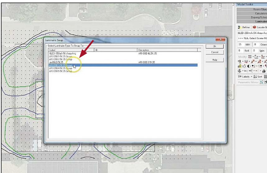
(32) When the Luminaire Swap Box pops up on the screen, click on the Group file that corresponds to the Composite file in the layout we are working on ...
