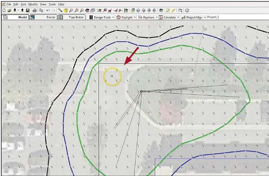
(38) As you do so, notice how the isolines dynamically calculate the foot-candle values as you aim each individual module. **And check this out. You can even aim or direct the light behind the pole,** hitting corners that would normally mess up your average or minimum foot-candle ratio, or to areas that you would normally need to add another luminaire!
