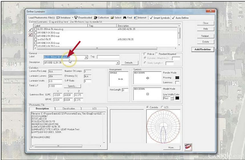
(23) The top file, 6LED-350mA-Avg, consists of an individual LEAR module file which is 6.77W and 699 lumens. As a very important note, **do not use this file in your layout. If you select this for your layout, it will calculate for only one module!**
