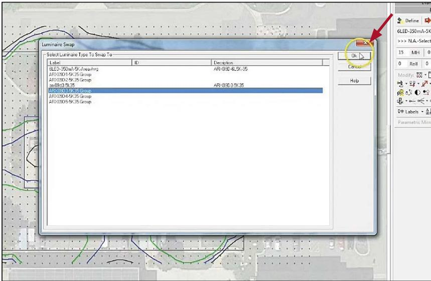
**(32a)** and click Ok. Just to reiterate, the Composite file we are using here is a 9 module 3X3, Type 3, 5000K, 350mA IES file which reads as, "ARX09D3-5K35". The Group file you choose here needs to correspond with that.
