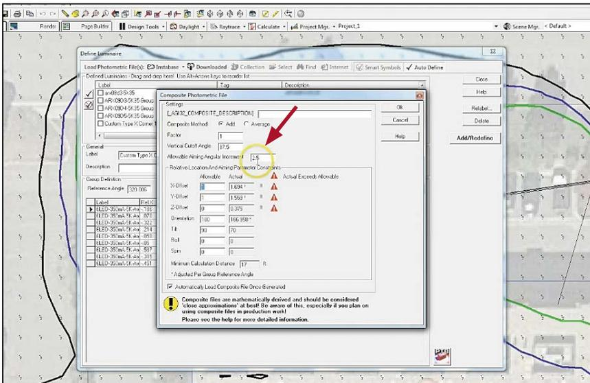
(50) Now, set the "Allowable Aiming Increment" to 2.5°. This just represents the tolerance on the angular increments in production.
