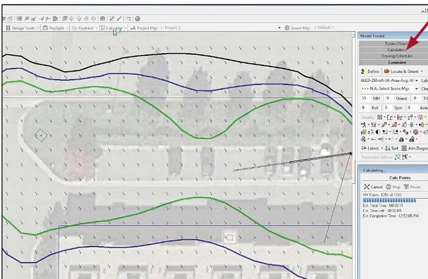
(61) Finally select calculations to run calculations for the layout.
