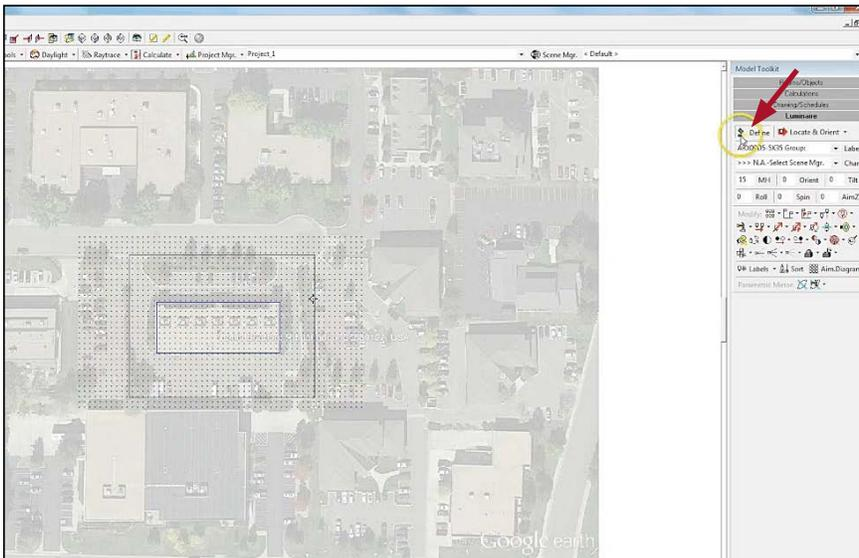
(21) Next, click on the “Define” button under the “Luminaire” tab at the top right of the screen.
