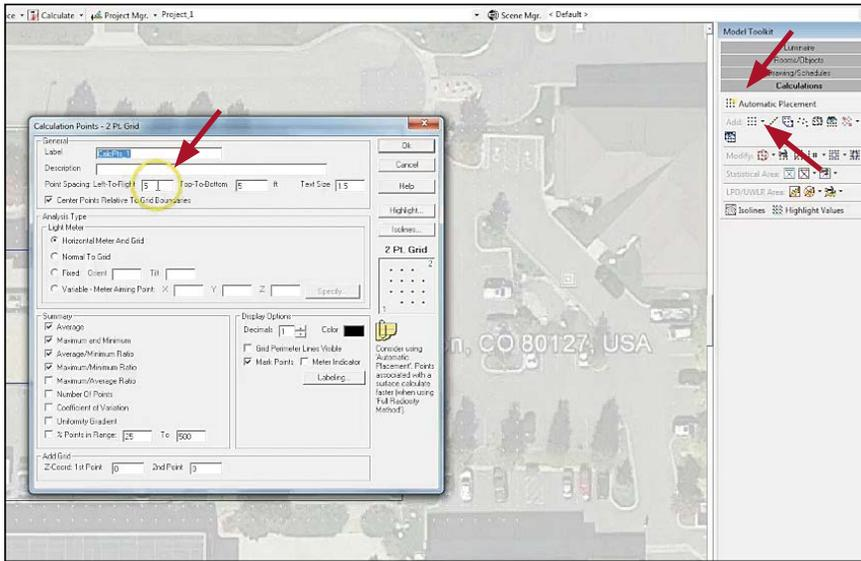
(4) Next, click on the Calculations Tab and add a 2 point grid. This is where you set the point spacing as required for your layout. In this case, we are choosing a 5 ft by 5 ft grid.
