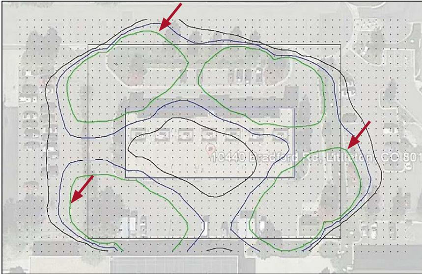
(30) As you can see, the standard Composite IES file is not “tailor fit” to the layout and there are some “light trespass” issues. At this point, this is where you would normally begin to move luminaires around, add fixtures, and add poles where needed, to place the light in the spots you want. Sound familiar?
