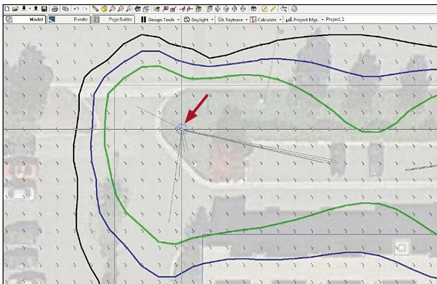
(42) Next, click on the group to define the insertion point and click a second time in the direction the fixture is oriented at to define the reference angle.
