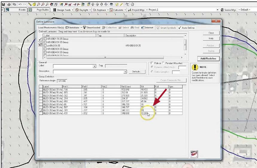
(44) Here you want to make sure that the individual module tilt is restricted to 70°, as that is the maximum angle the LEAR module can vertically rotate.
