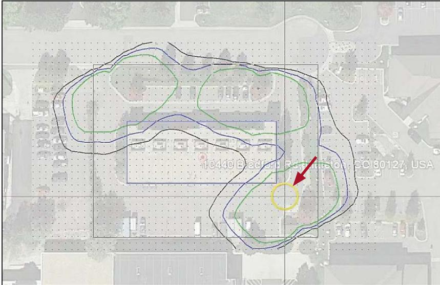
**(28)** Notice as you continue to add luminaires to the layout, the Design Isolines dynamically calculate with one another.
