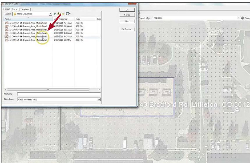
(19) In this example, we are going to import the 9 module 3X3-350mA-5K-Import\_AreaFinal, so, click on the file and select “Ok”. As a side note, if you are working with a “metric” layout, you will want to choose the file with “metric” in the file’s description.
