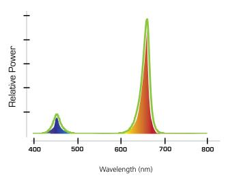
The Partial-spectrum Vegetative mix (V1), provides only red and blue wavelengths conducive to photosynthesis. V1 is designed for the vegetative growth stage of plant life, and is considered robust enough to support the entire plant growth cycle, if desired.
