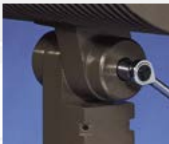
Both the standard swivel and Heavy Duty Swivel (HDS) option shown here are easily adjustable
