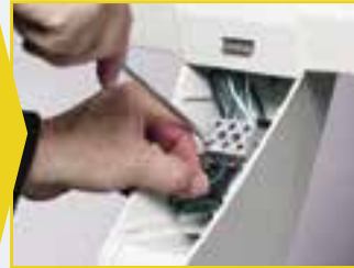
CONNECT WIRES TO TERMINAL BLOCK
