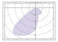
20L-Cx-35K-D075-PR-04-D10 with Parabolic Wall/Slot° 2000 LED, 4', 3500K, 750 lum/ft, 11W/ft, matte white finish, upper parabolic reflector, 0-10V dimming driver at 100% output
