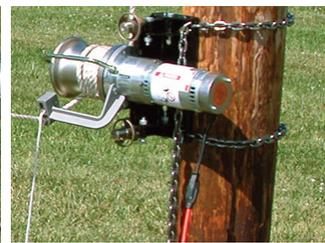
**Optional Rope Lock** – At left: Automatically supports load when fall line is released, until operator resumes hoisting. At right: The release lanyard permits lowering or lifting load with precise control over speed and distance.
