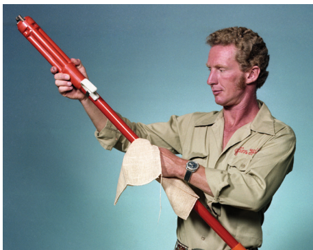
Cleaning a pole with Chance Moisture Eater II
