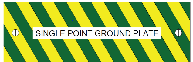
FAA4 = SINGLE POINT GROUND PLATE* Alternating Green and Yellow stripes
