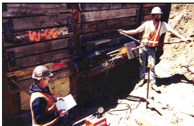
ANCHOR TENSION LOAD TEST IN MINNEAPOLIS, MN FIGURE B-2
