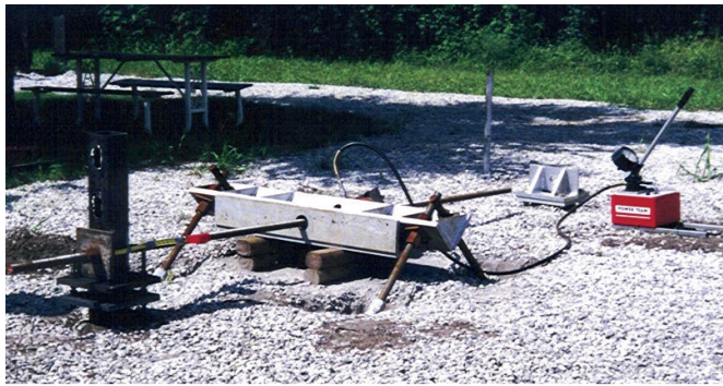
LATERAL LOAD TEST APPARATUS FIGURE B-6
