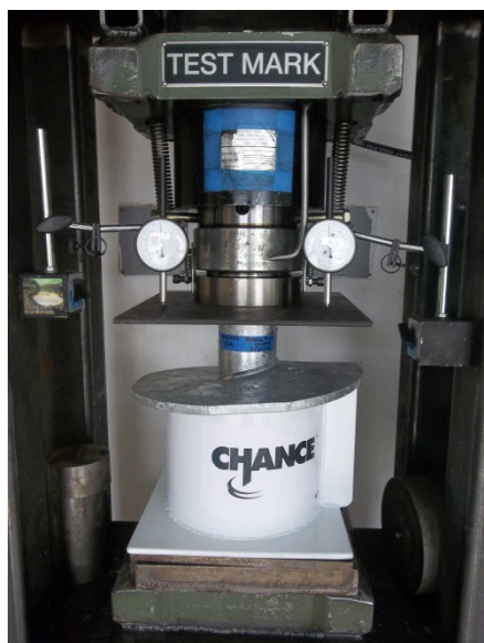
FIG. C-1 – P3 HELIX STRENGTH SET-UP
