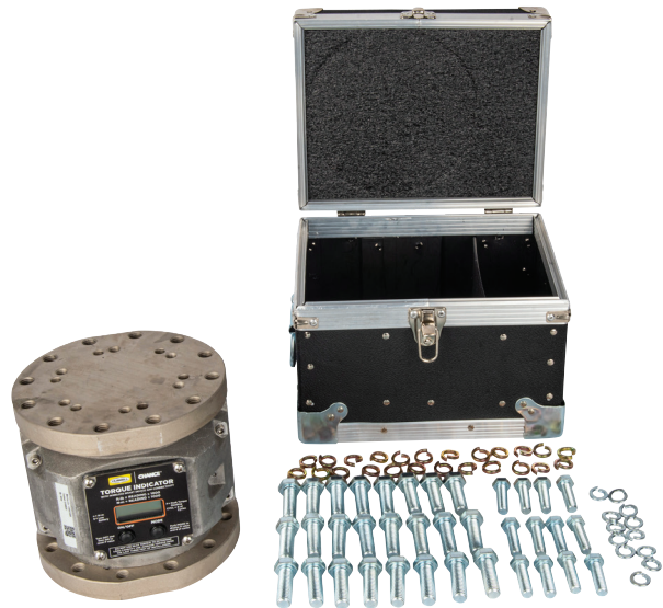
Digital Torque Indicator with Included Case and Hardware, Figure 5-11
