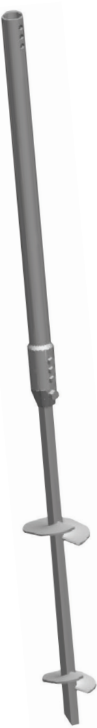
Pile Assembly with Transition Coupler Figure 6-45
