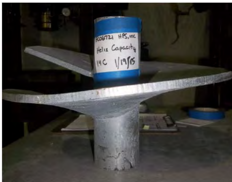
FIG. C-2 – RS2875 14" DIA. HELIX - TEST RESULTS
