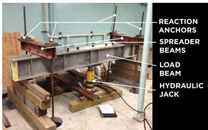
INDOOR COMPRESSION TEST FIGURE B-4
