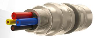
The RCG Coupler provides the means to extend an existing cable without the need to use a junction box, or a more permanent splice kit. Combining two RCG cable glands and a simple termination system makes upgrading installations fast and easy.
