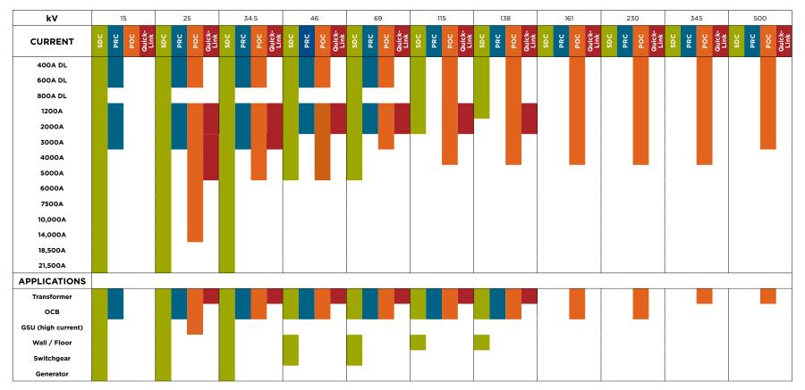
SDC® - Solid-Dielectric-Capacitor Type, cast epoxy composite bushing, capacitance graded, oil-free.
