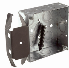
Box-Loc® "MS" Bracket Positions box on either side of stud. BOX-LOC® (MS) Bracket Box is a snap to install. Place the bracket on the open side of the stud first. Slots in the bracket engage the lip of the stud and actually crimp it as you press the bracket on the stud. Barbed hooks dig into the flat side of the stud, quickly locking it into place.
