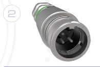
Integral Keying - Our machined keyway ensures perfect connector alignment without damage to pins or contacts for fast installation and a longer product lifespan. The 5 positions for OP-PR and a unique 6<sup>th</sup> position for OP-IS prevents cross-mating between two protection concepts.
