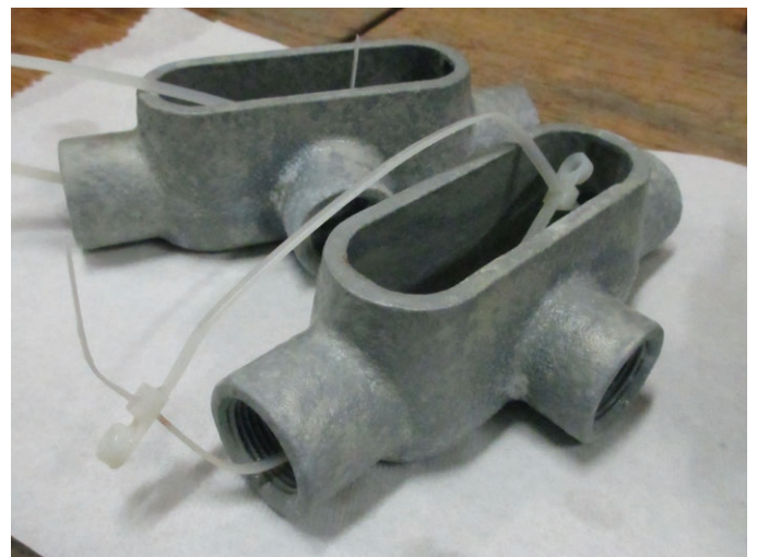
Representative samples of new Duraloy ® Plus paint after 1,000 hours of exposure
