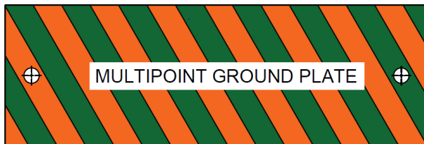
FAA3 = MULTIPOINT GROUND PLATE* Alternating Green and Orange stripes
