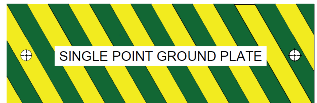
FAA4 = SINGLE POINT GROUND PLATE* Alternating Green and Yellow stripes
