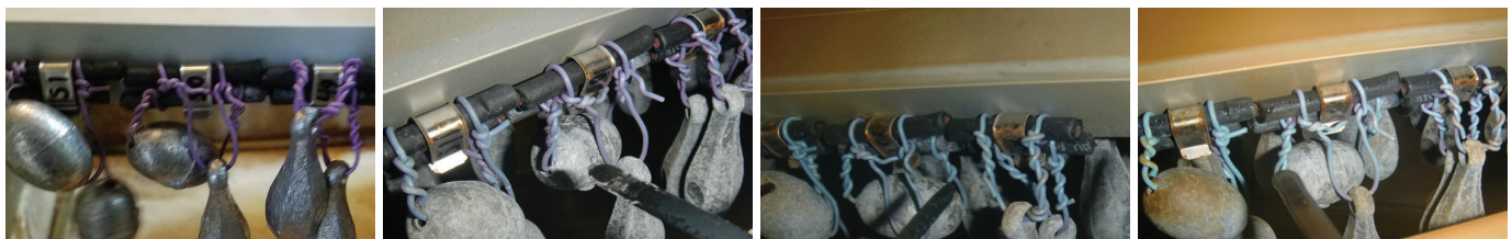
Figure 4 - Increasing material degradation at setup, 532 hrs, 1028 hrs, and 1540 hrs (left to right)
