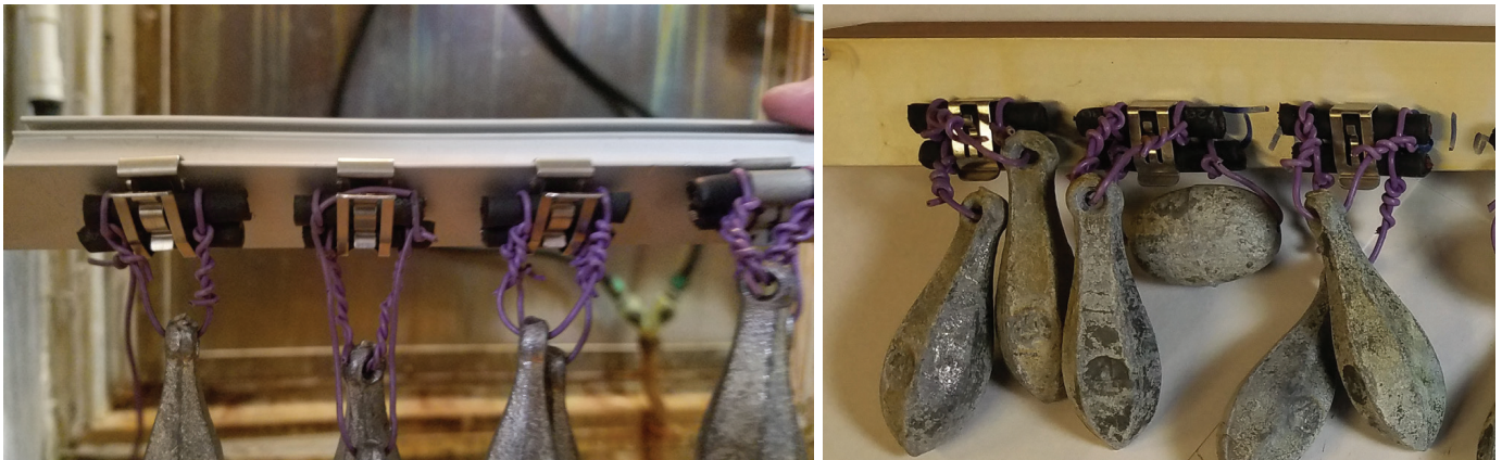
Figure 5 - Wiley grade material pre- and post-test with no visible degradation
