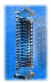
Powerohm offers replacements for roof mounted braking resistors on buses, utilizing punched grid elements for superior cooling over the round edgewound elements furnished by the O.E.M. The flat surface of the grid element allows air to flow over a larger surface area, more effectively cooling the element, reducing fatigue and increasing longevity.
