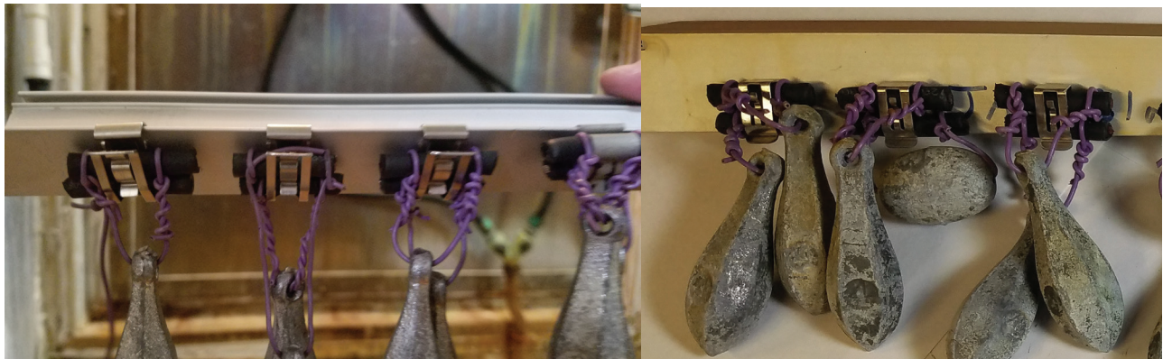
Figure 5 - Wiley Grade Material Pre- and Post-Test with No Visible Degradation
