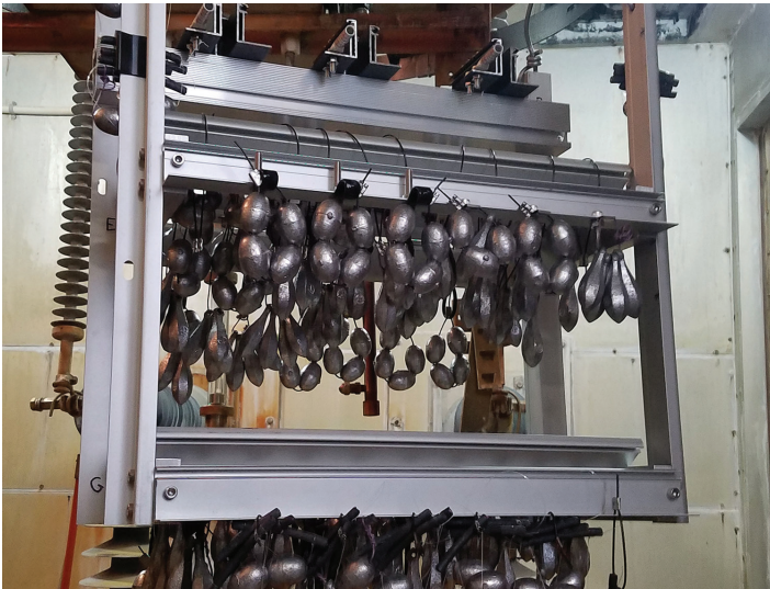
Figure 3 - Test Fixture Installed in Environmental Chamber
