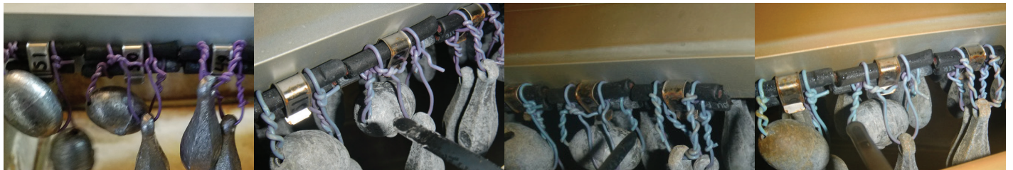
Figure 4 - Increasing Material Degradation at Setup, 532 hrs, 1028 hrs, and 1540 hrs (left to right)
