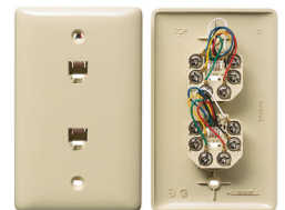
Duplex RJ11 Jacks, 6-Position, 6-Conductor, Screw Terminations
