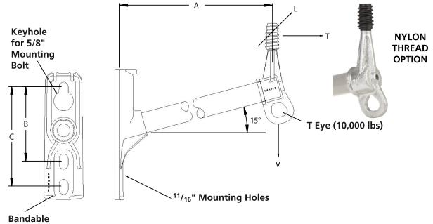
B Dimension is 6" for 1SBM series and 8" for 1SBH series C Dimension is 8" for 1SBM series and 10" for 1SBH series
