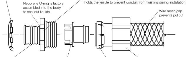
Insulated throat protects insulation on wires during pulling; yellow color easily seen by inspectors Yellow nylon ferrule fits inside nonmetallic conduit to hold the shape; barb in designed to assure liquidtight seal even with non-square cut; ferrule is keyed to fit into body to prevent conduit twisting Hexagonal compression nut is machine steel through 1" malleable iron on larger sizes; tapered interior compresses sleeve over conduit sealing out liquids and preventing pullout
